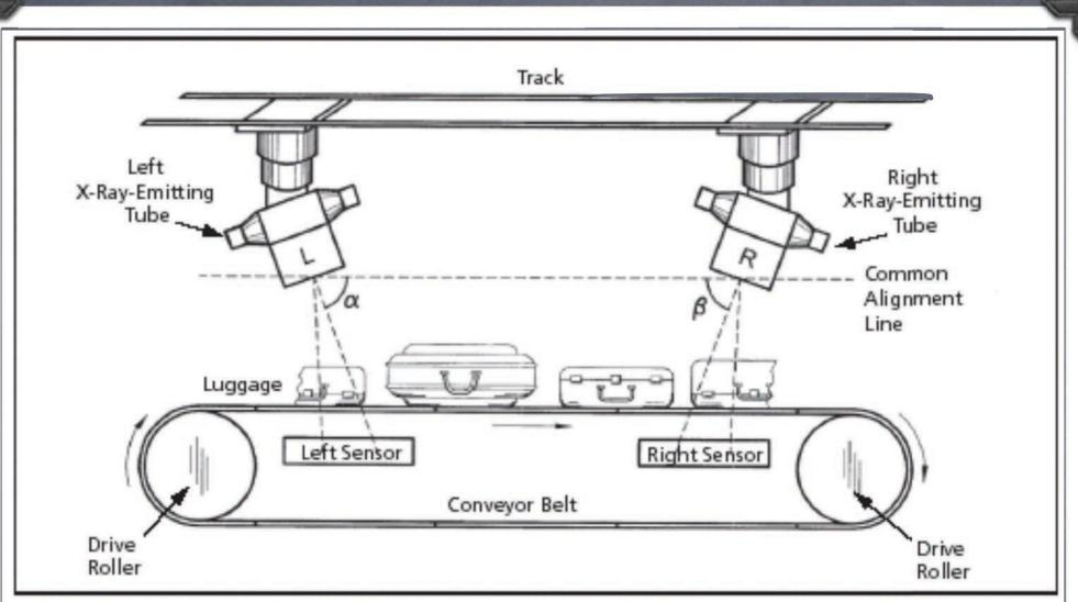
Images From the Left- and Right-Eye X-Ray Sensors are captured at different locations and stored along with conveyor position data allowing the appropriate left- and right-eye images to be viewed by the human operator on a commercially available stereo display screen.
