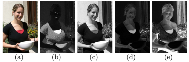
Figure 2: Cylindrical coordinate color space. (a) Color image; (b) hue; (c) brightness; (d) non-normalized saturation. For comparison (e) saturation using the HSV conversion formulae.
