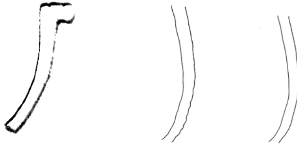
Figure 4: (a) acquired profile - (b) spline (c) smoothed spline
