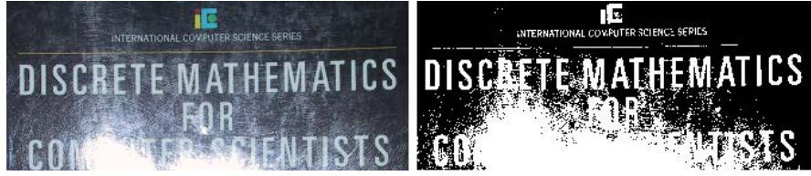
Figure 2.1: Segmentation errors caused by binarizing the image with Otsu [66].
