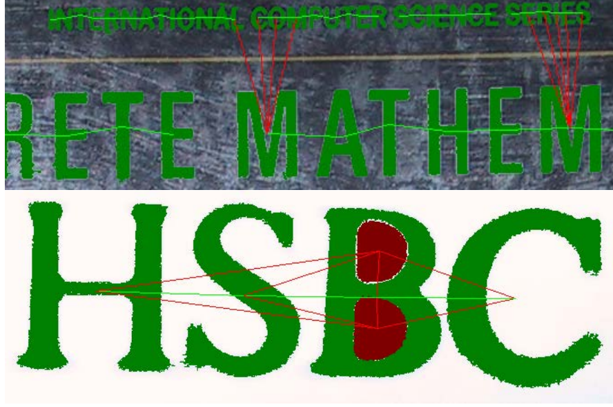
Figure 3.17: Adjacent text-CCs in the same textline are positive cases (top and bottom), adjacent text-CCs in different textlines (top) and adjacent text and non-text CCs (bottom) are negative cases.
