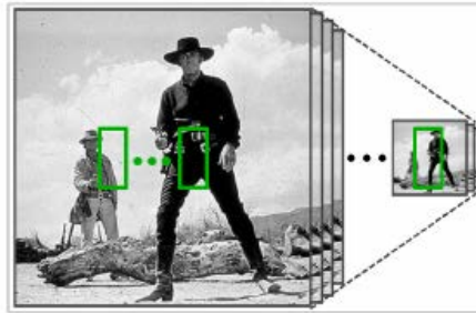
Figure 2.4: Sliding window detection for pedestrians proposed by Dollar et al. [20]
