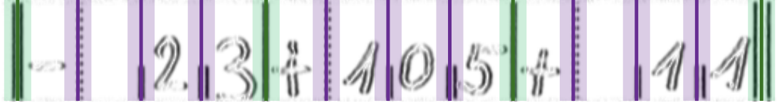
Figure 3.8: Absolute horizontal gradient image |f_x| for one row in the ROI with the search areas for the precise frame line localization defined by the global (green) and local (purple) lines in the reconstructed form and a \pm 9 pixel margin.
