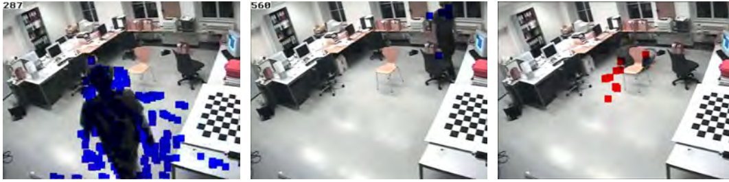
Abbildung 1.8: Results of the Cosamed project. Rectangles are placed on temporal centers of detected features. Blue are features of usual behavior, red gives emergency feedback classified by a Mahalanobis nearest neighbor classification of clustered local 3D jets.
