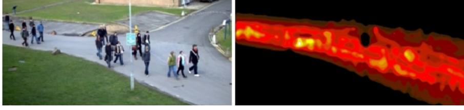
Figure 4.13: Input image (left) and the corresponding trained accumulated hitmap (right) [ZK10].
