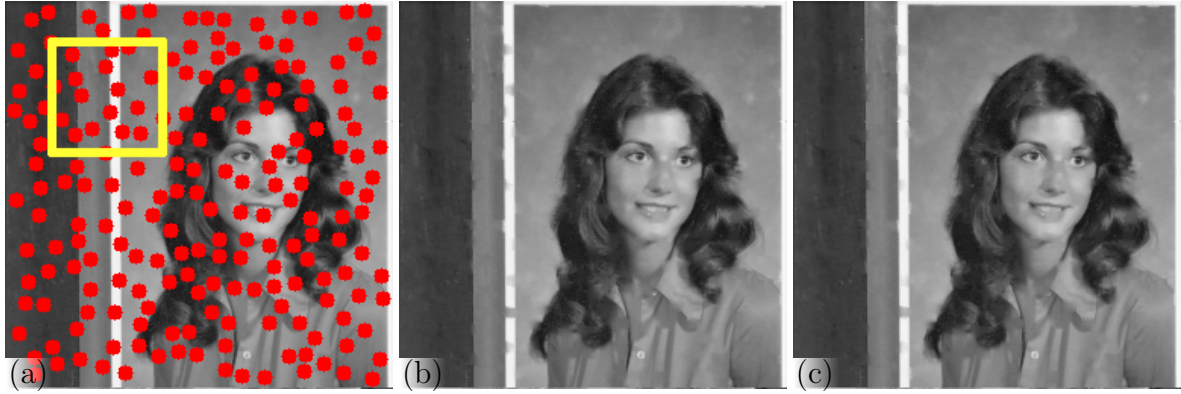
Figure 4.7: Inpainting of the circle mask, shown in (a). (b) Black initialization result: PSNR = 33.54 dB. (c) Mean initialization result: PSNR = 34.30 dB.
