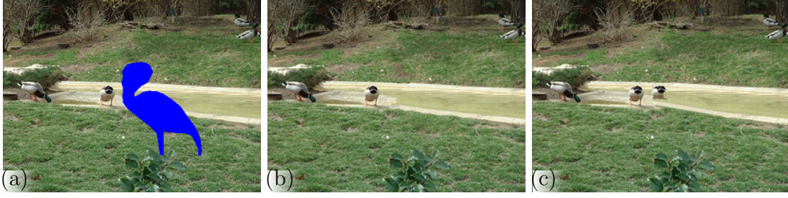
Figure 2.13: Comparison of two exemplar-based methods. (a) Input image with overlying mask (blue). (b) Outcome of the extended algorithm proposed by Zhou and Robles-Kelly. (c) Output of the basic exemplar-based algorithm published by Criminisi et al. It is obvious that the basic algorithm produces artifacts, which are avoided by the extended version. [ZRK10]
