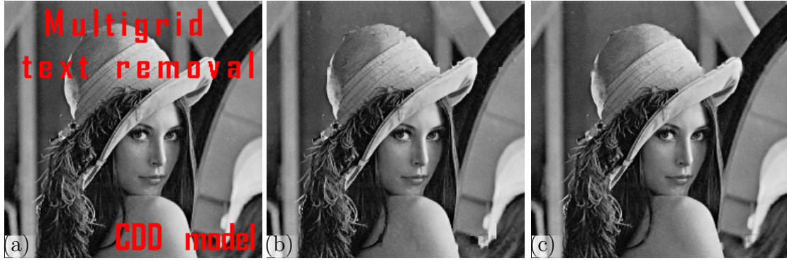
Figure 4.12: Text removal example. (a) Lena image and inpainting mask (b) Result obtained by the TV based algorithm in [BLC08]. (c) Image inpainted with the help of an FOE prior.
