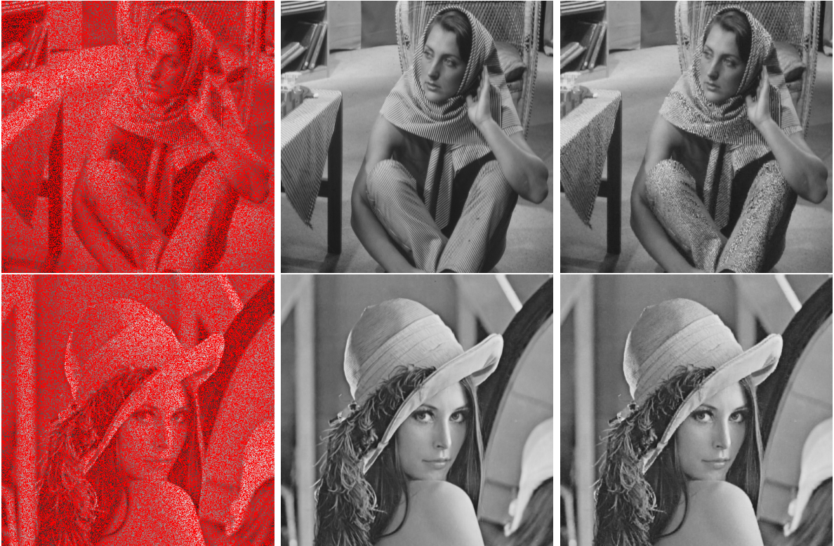
Figure 4.14: Inpainting of a randomly generated mask. (Left) Input images with superimposed masks. (Middle) Resulting images produced by the method in [YSM10]. (Right) Images recovered with an FoE prior.
