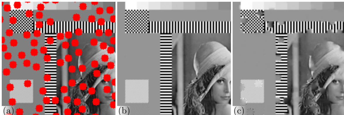
Figure 4.6: Limitation of the inpainting algorithm. (a) Input image. (b) Ground truth image. (c) Image inpainted with \eta = 110 . The PSNR value of the inpainting result is low, namely 24.93 dB.
