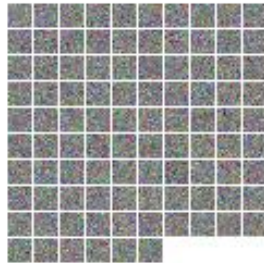
Figure 5.7: Random initial values for weights of the first convolutional layer are sampled from a Gaussian distribution.
