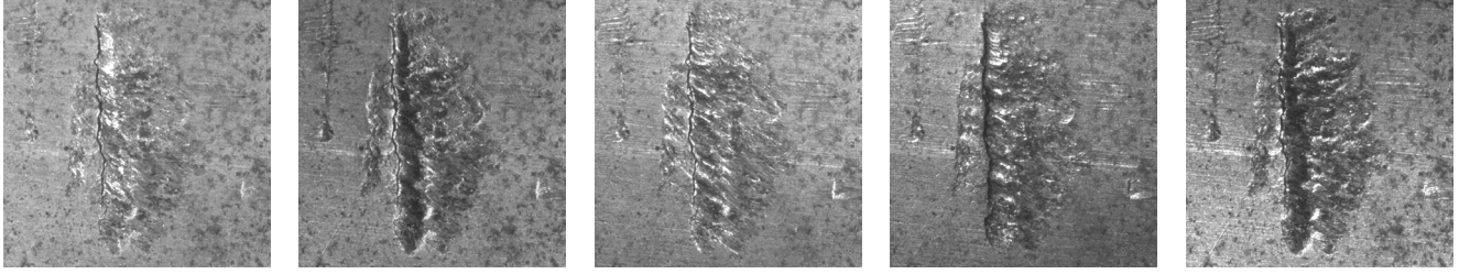
Fig. 3: Toolmark crop under different lighting conditions.
