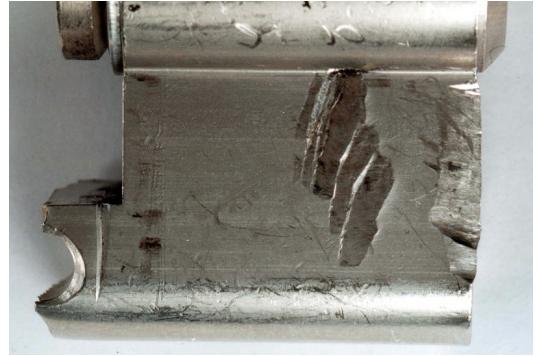
Fig. 1: Snapped lock with multiple toolmarks.
