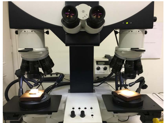
Fig. 2: Leica comparison microscope used by the forensic experts in Austria.
